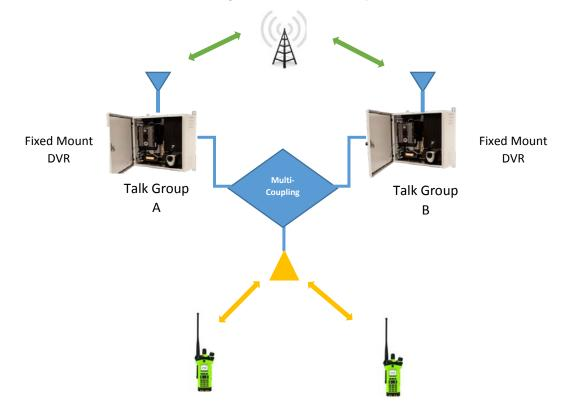
While being significantly less expensive than a full site, there are some limitations with the DVRS. The users need to switch channels to a conventional channel, but this is a small price to pay to obtain radio coverage. Using DVRS enabled subscribers on a P25 Trunking system, most key P25 features are available. These include PTT and emergency ID pass through, network affiliation, OTAR, patch, end to end encryption, end to end digital audio and stun/kill.
