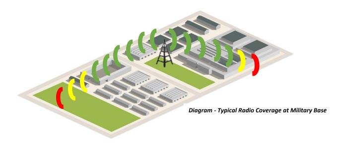
In many remote areas, mobile radio coverage may not be available as a result of terrain or distance for a tower site. Adding radio sites for these situations may not be practical or economically feasible. For a number of these situations, fixed mount DVRS have provided a solution. Missile sites in mountainous regions, range control, chemical and weapons storage areas and remote buildings are a few examples where the DVRS has been deployed.
