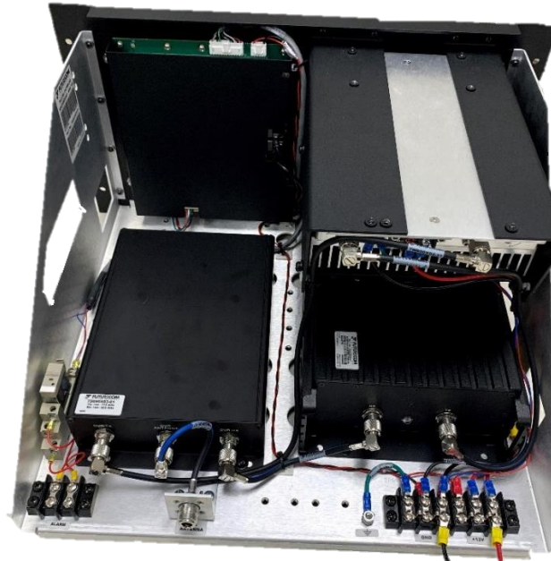
Figure 12: Rackmount PDR8000 Back Panel
