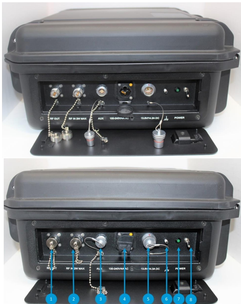
Figure 31: Booster Pack External Ports
