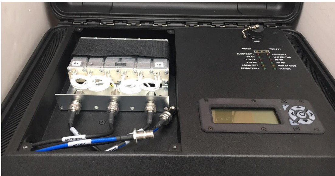
Figure 3: Internal Duplexer Cavity
