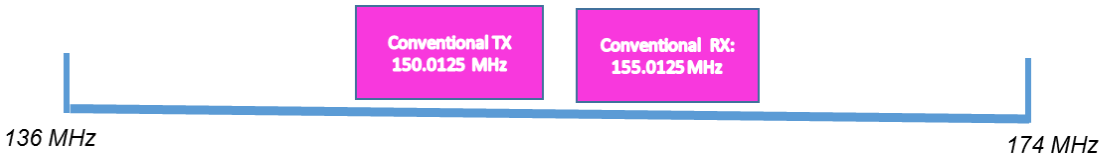
Figure 13 – Conventional VHF System Frequencies
